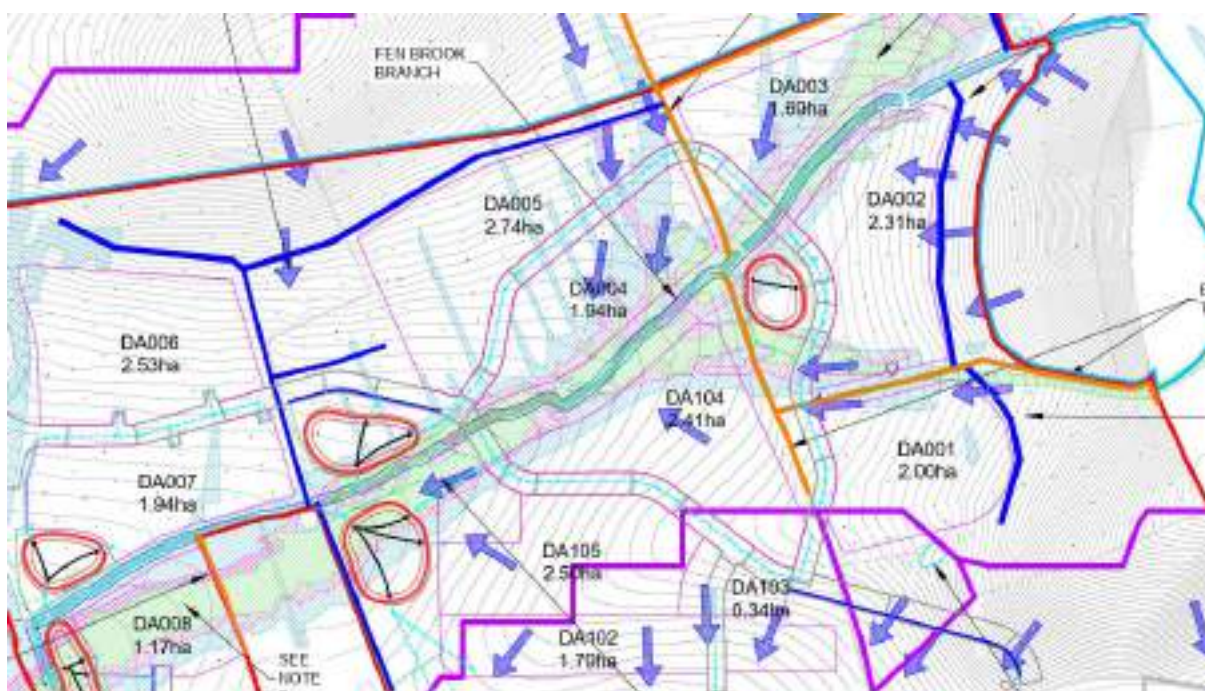
Figure 4 Pluvial flood risk and overland flow routes
