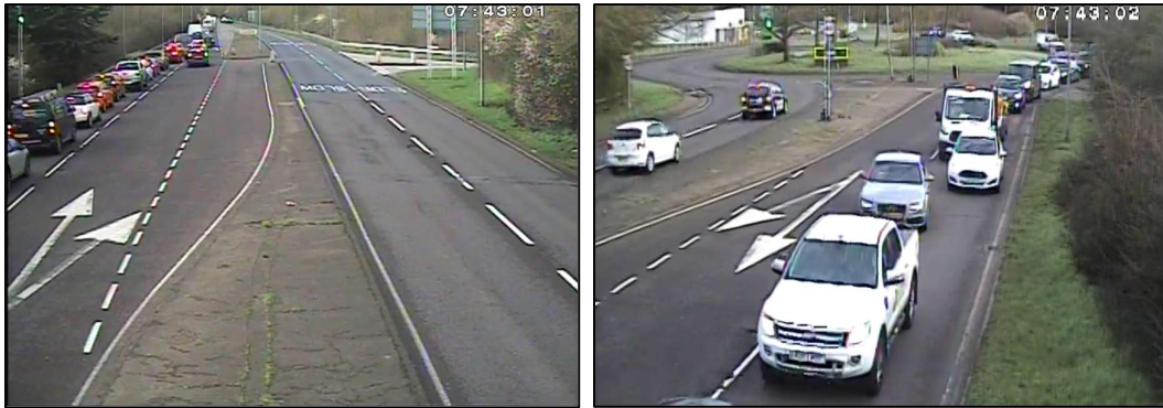
Figure 7.4: Queuing on Burnham Road Due to Narrowing From 2 lanes to 1 lane
